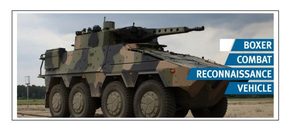
The Army is getting a new Combat Reconnaissance Vehicle (CRV) to replace the ASLAV which is being withdrawn due to its inadequate blast protection. Two hundred and eleven (211) Boxer CRV's, are presently being built at Ipswich QLD by Rheinmetall. The Boxer has very good kinetic blast protection and sports a 30 mm cannon, 7.62 mm MG, a 12.7 mm Remote Weapon Station and an Anti-tank Guided Missile System. Maximum speed is 103 kph. The Boxer CRV will be in service by 2020.
